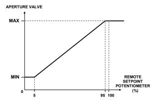
Aperture setting MIN : Set the setpoint potentiometer in min stop (Stop when potentiometer turn in reverse clockwise). Set minimal aperture with MIN potentiometer on the rear panel.
