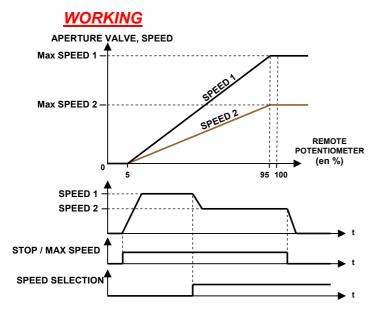
Setting the speed 1 (Pot MIN): Do not shunt the "SPEED SELECTION" input with +POWER, set the setpoint potentiometer to the maximum stop (stop when turning the potentiometer clockwise) and "STOP / MAX SPEED" switch to ON. Set speed 1 with the MIN potentiometer on the rear panel.
