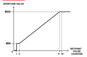
10 pulses on input PLUS are required to open the valve from minimum to maximum. 10 pulses on input LESS are required to close the valve from maximum to minimum.
