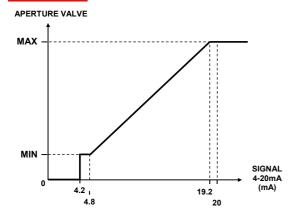
Aperture setting MIN: Set 4-20mA signal to 4.5mA. Set minimal aperture with MIN potentiometer on the rear panel.
