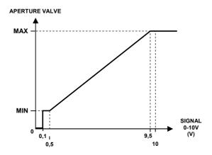
Aperture setting MIN: Set 0-10V signal to 0.3V. Set minimal aperture with MIN potentiometer on the rear panel.
