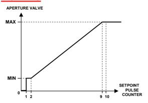
10 pulses on input PLUS are required to open the valve from minimum to maximum. 10 pulses on input LESS are required to close the valve from maximum to minimum.
