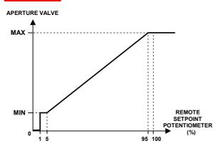
Aperture setting MIN: Set the setpoint potentiometer to 0 (Stop when potentiometer turn in reverse clockwise). Then turn it slightly in the opposite direction until the LED blinks. Set minimal aperture with MIN potentiometer on the rear panel.
