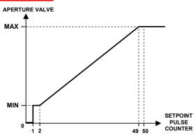
50 pulses on input PLUS are required to open the valve from minimum to maximum. 50 pulses on input LESS are required to close the valve from maximum to minimum.
