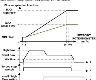
Aperture setting MIN: Set the setpoint potentiometer to 0 (Stop when potentiometer turn in reverse clockwise). Then turn it slightly in the opposite direction until the LED blinks. Set minimal aperture with MIN potentiometer on the rear panel
