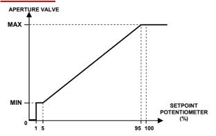
Aperture setting MIN: Set the setpoint potentiometer to 0 (Stop when potentiometer turn in reverse clockwise). Then turn it slightly in the opposite direction until the LED blinks. Set minimal aperture with MIN potentiometer on the rear panel
